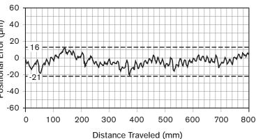
Regardless of the distance traveled, positional accuracy remains constant with the RPS System.
